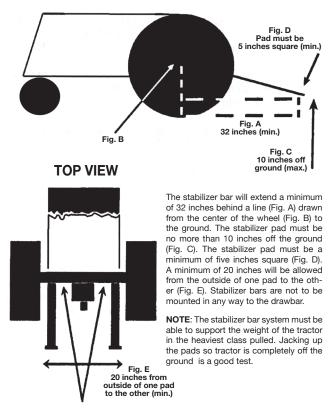
The stabilizer bars and their assembly are in no way to be connected to the drawbar or its assembly.
